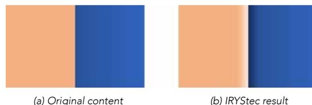
Figure 1 shows a simple example of how IRYStec's image processing enhances contrast locally. In (a) the original content is shown: simple border between two regions of different color; (b) shows the original image with IRYStec's enhancement of contrast. Notice how the near-boundary pixels are modified: the brights are brighter, whereas the darks are darker; overall, the processed image has more contrast near boundary.
