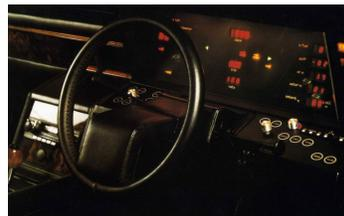
Figure 2: Aston Martin Lagonda electronic instrument cluster, 1976
